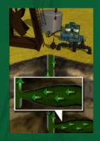
NuFlo™ chemical injected downhole breaks down paraffin and asphaltene deposits that have accumulated over time; fluid flow increases and formation returns to free-flowing state at full reservoir potential.
